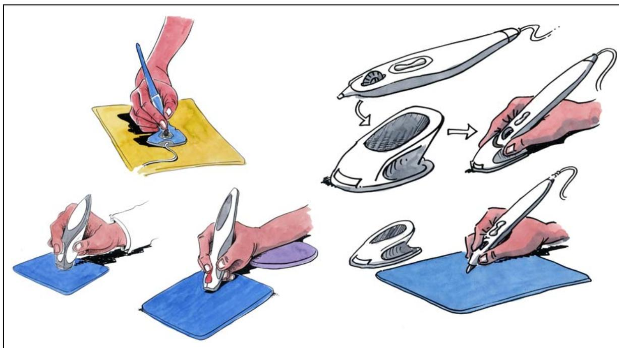
Other mouse shapes that displayed positive effects on posture and muscle activity in comparison to conventional mouse designs tended to be larger, adapted to the contours of the hand – in part individually by way of gripping the device – and swept outward (towards the ulna) in order to reduce forearm pronation [51; 62]. Figure 22 shows examples of such mouse designs.
