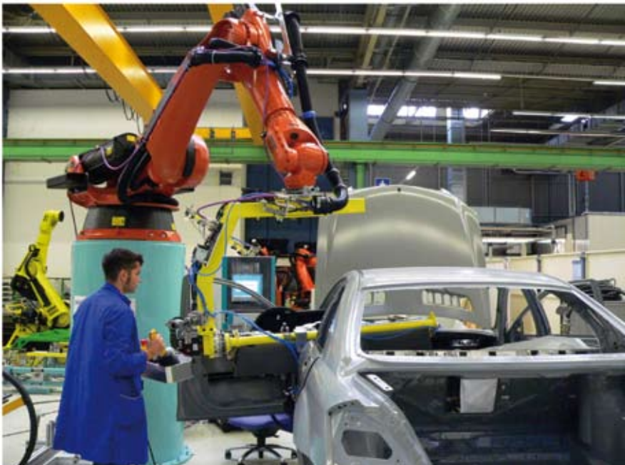
Fig. 2: Dashboard assembly, Source: Daimler AG
