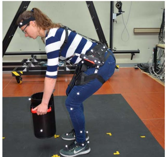
Experimental setup for testing exoskeletons in the laboratory
