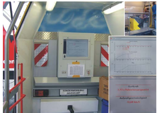
Acceleration measuring device with details of measured signals and data
