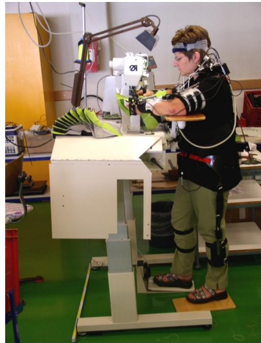
The newly developed ergonomic sewing workplace; sewing operative fitted with the CUELA measurement system
