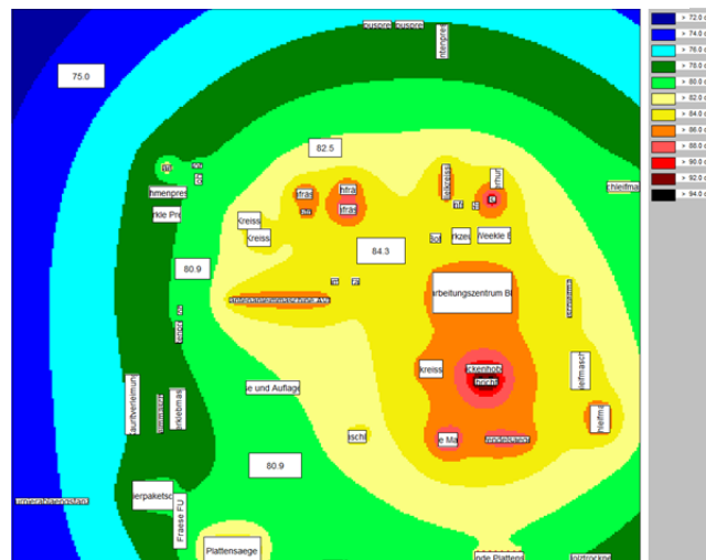
Sound pressure level distribution calculated to VDI 3760 for a woodworking company
