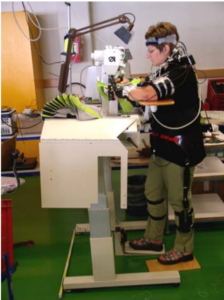
Figure: The newly developed ergonomic sewing workplace; sewing operative fitted with the CUELA measurement system
