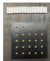
Figure 1: ASTM F2010 test apparatus
