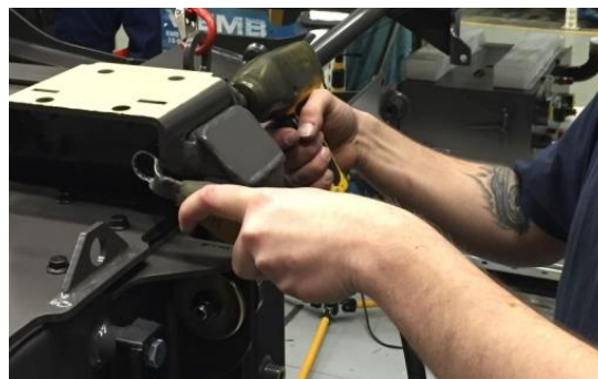
Figure 1: Assembly with impact wrench and anvil.
