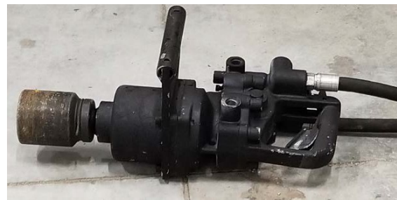
Figure 1: Impact wrench used for track/rail bolts in the railway maintenance-of-way industry
