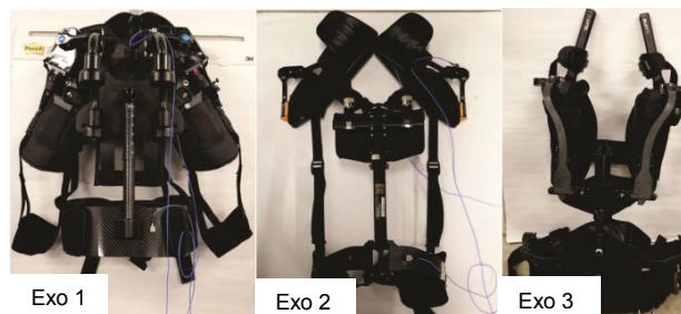
Fig. 1: Three exoskeleton vest models were evaluated in this study. The vests are adjustable to accommodate a wide variety of body shapes and sizes. Each exoskeleton model has multiple spring settings that allow the exoskeleton to provide various levels of mechanical assistance to the worker.
