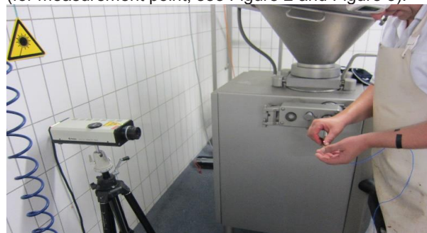
Figure 3: Reference measurement with laser vibrometer
