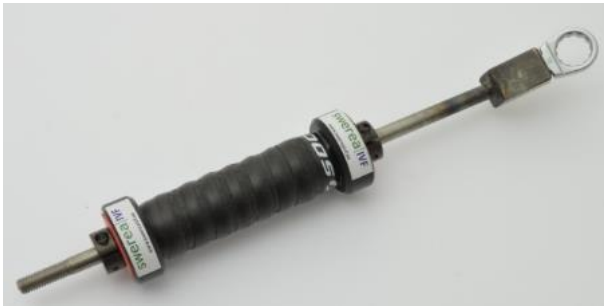
Figure 2: Vibration isolated anvil
