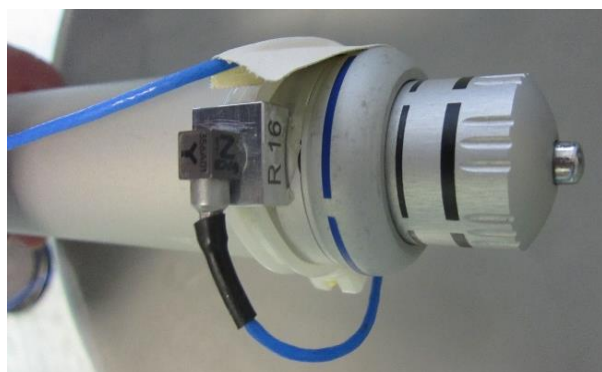
Figure 2: The attachment of the sensor on a shockwave therapy tool
