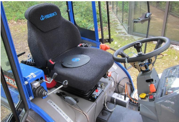
Figure 3: Attachment of the devices for measuring a) HAV and b) WBV
